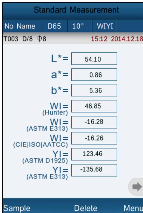
Figure 25 LAB & WI & YI Standard Measurement
