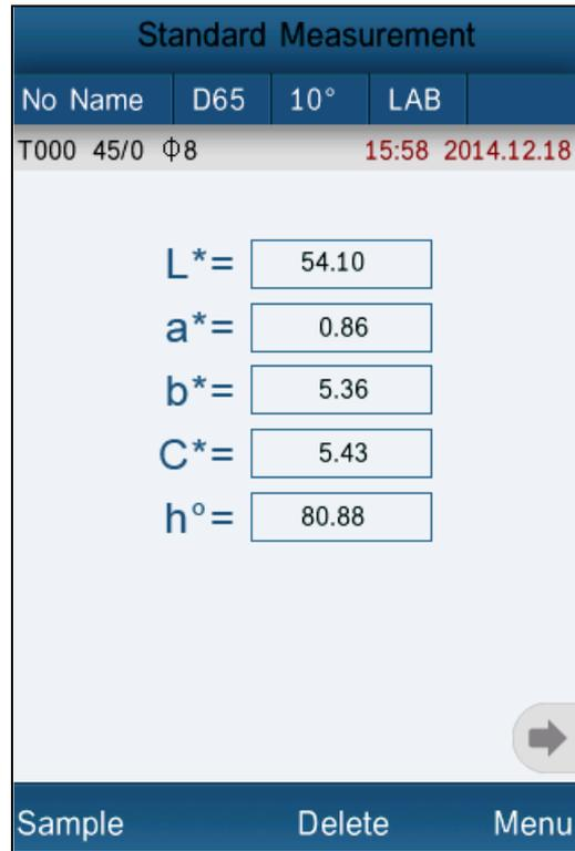
Figure 3 Standard Measurement
